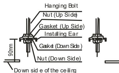
Install the hanging bolt into T groove of the hanging tool. Overhang the indoor unit and ensure it is level using a level indicator.
