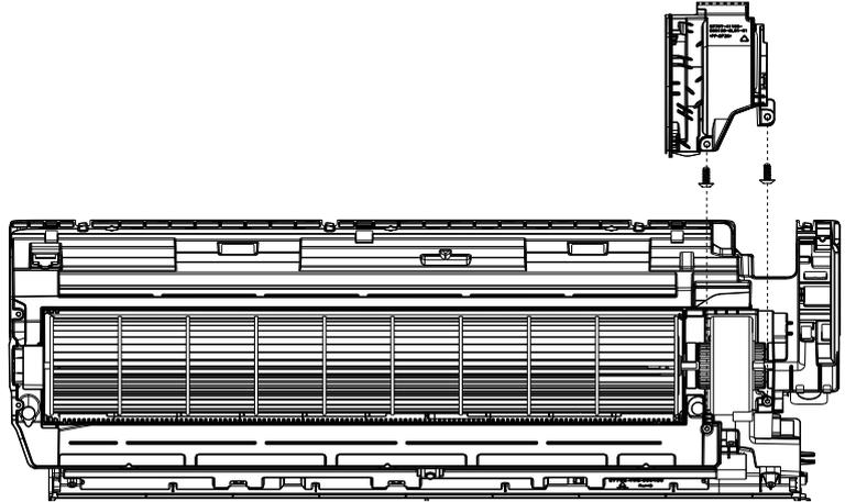
**12. Disassemble Fan motor and Cross fan**
