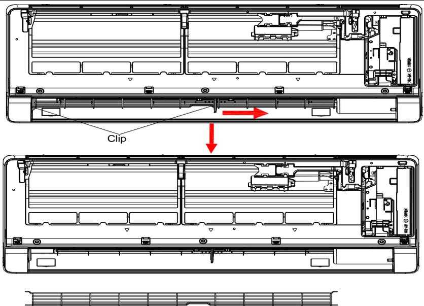
**7. Disassemble the middle Frame.**
