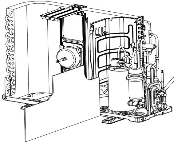
**step7: Disassemble the separate plate**
