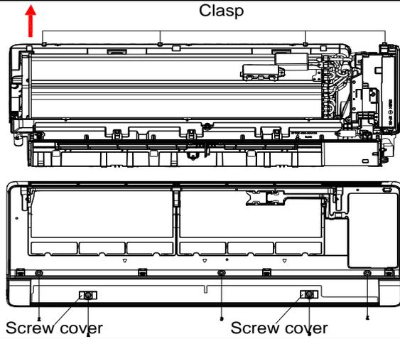
**8. Disassemble the Electric control box.**
