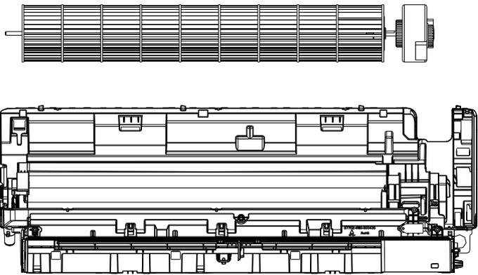
**13. Disassemble Cross fan from Fan motor**
