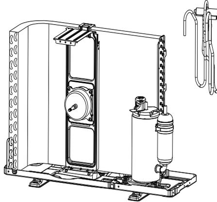
**step10: Disassemble the compressor.**
