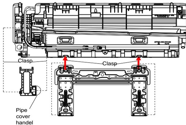
**10. Disassemble the Evaporator**
