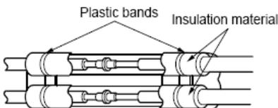
Wrap the area which accommodates the rear piping housing section with vinyl tape.
