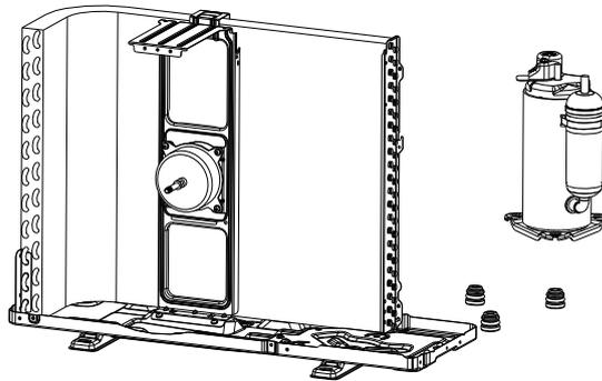
**step11: Remove the fan motor and fan supporter**
