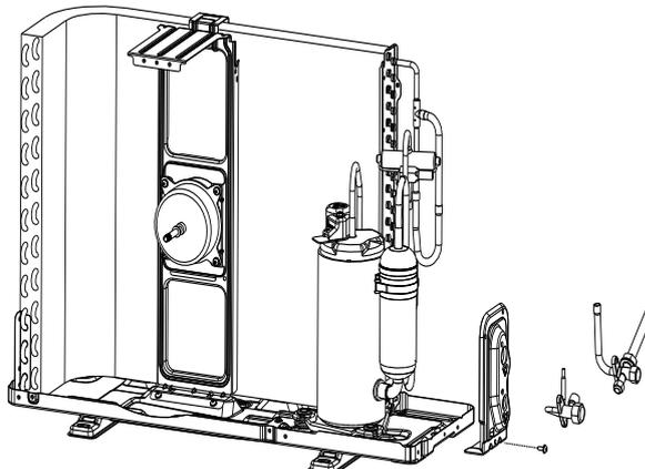
**step9: Disassemble the 4-way valve assembly**
